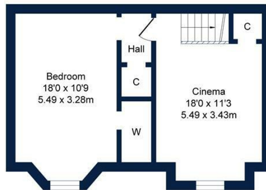
Lower Ground Floor Approx. Floor Area 437 Sq.Ft (40.6 Sq.M.)
